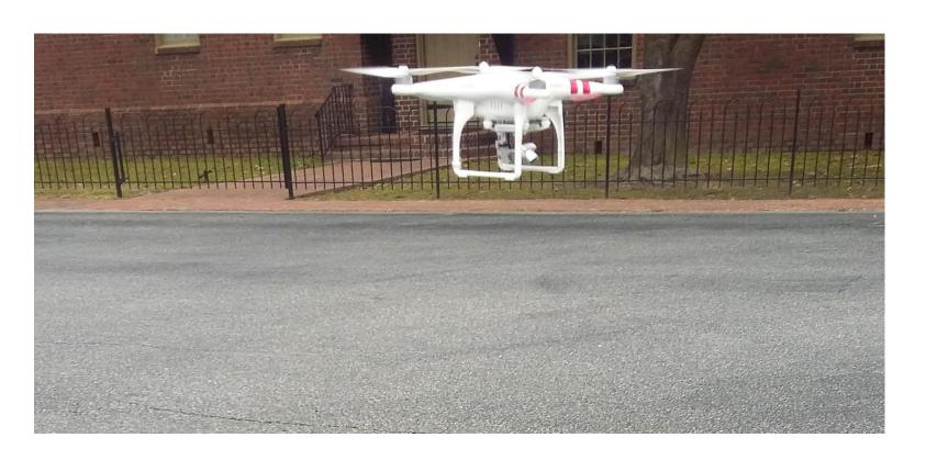
The primary piece of equipment used to conduct this research was the DJI Phantom 2 Vision+ U.A.V. with a built-in NazaM V2 Flight Control System and integrated gimbal and camera (Fig. 5) [1]. The Phantom 2 Vision+ is a two pound remote-controlled quadcopter that contains four rotating wings capable of stable flight and taking high resolution pictures and video.
